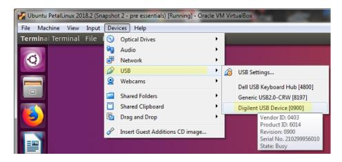
Once the device is detected and enumerated under Ubuntu, the USB-UART port should be listed under one of the /dev/ttyUSBx device entries. Locate the device entry for the USB-UART and make a note of this device for use in a later step.
