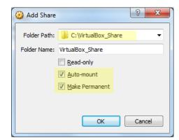
4. The location of the shared folder in Windows is shown in the Path column. The folder will Auto-mount and Full Access is allowed. The corresponding folder in the Linux VM is /media/sf\_<Windows Folder Name>. In the example shown, this corresponds to:
